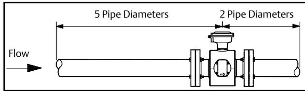
Consult the factory for performance in applications with less than ideal straight runs. Sensors can be installed with as few as zero diameters of straight run.
