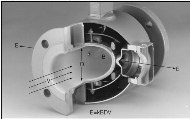
Magnetic field coils placed on opposite sides of the pipe generate a magnetic field. As the conductive process liquid moves through the field with average velocity  $V$ , electrodes sense the induced voltage. The width of the conductor is represented by the distance between electrodes. An insulating liner prevents the induced voltage signal from shorting to the pipe wall.
