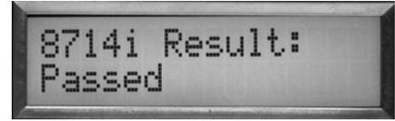
SMART Meter Verification checks transmitter and sensor characteristics.
