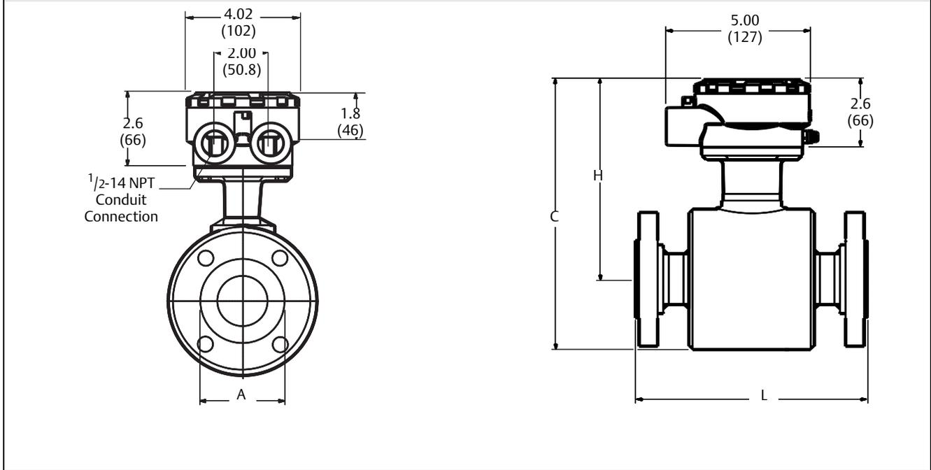
**Figure 9. Rosemount Flanged Sensors, typical of 6-in. to 48-in. (150 mm to 1200 mm) line sizes**
