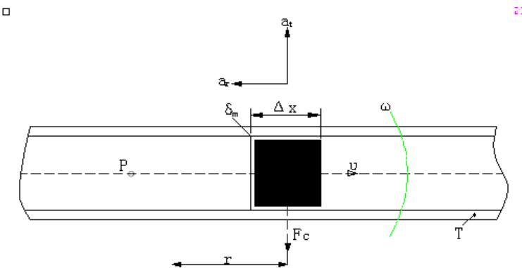
The measuring principle is based on the controlled generation of Coriolis Forces. Figure in the quality of the  $\delta m$  at a constant speed  $v$  of particles revolve around a fixed point  $P$  with angular velocity  $\omega$  movement of the pipe, the particle will receive two acceleration components:
